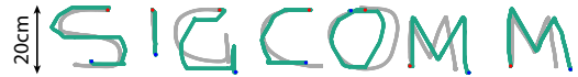
Figure 18: Examples of handwriting using RIM. The trajectories in green are estimates of RIM, while the gray ones are the ground truths captured by a camera.
